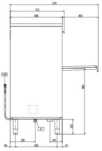
Drain EI = Electrical inlet (power) Electrical Outlet Hot water inlet
